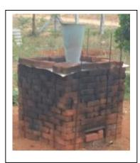
A similar experiment was done by taking less quantity of 15 kgs in a tin. This was heated for 1.30 hours and it was found to be perfectly converted to charcoal. It was understood that FS will burn and produce intense heat lasting for a long duration.
